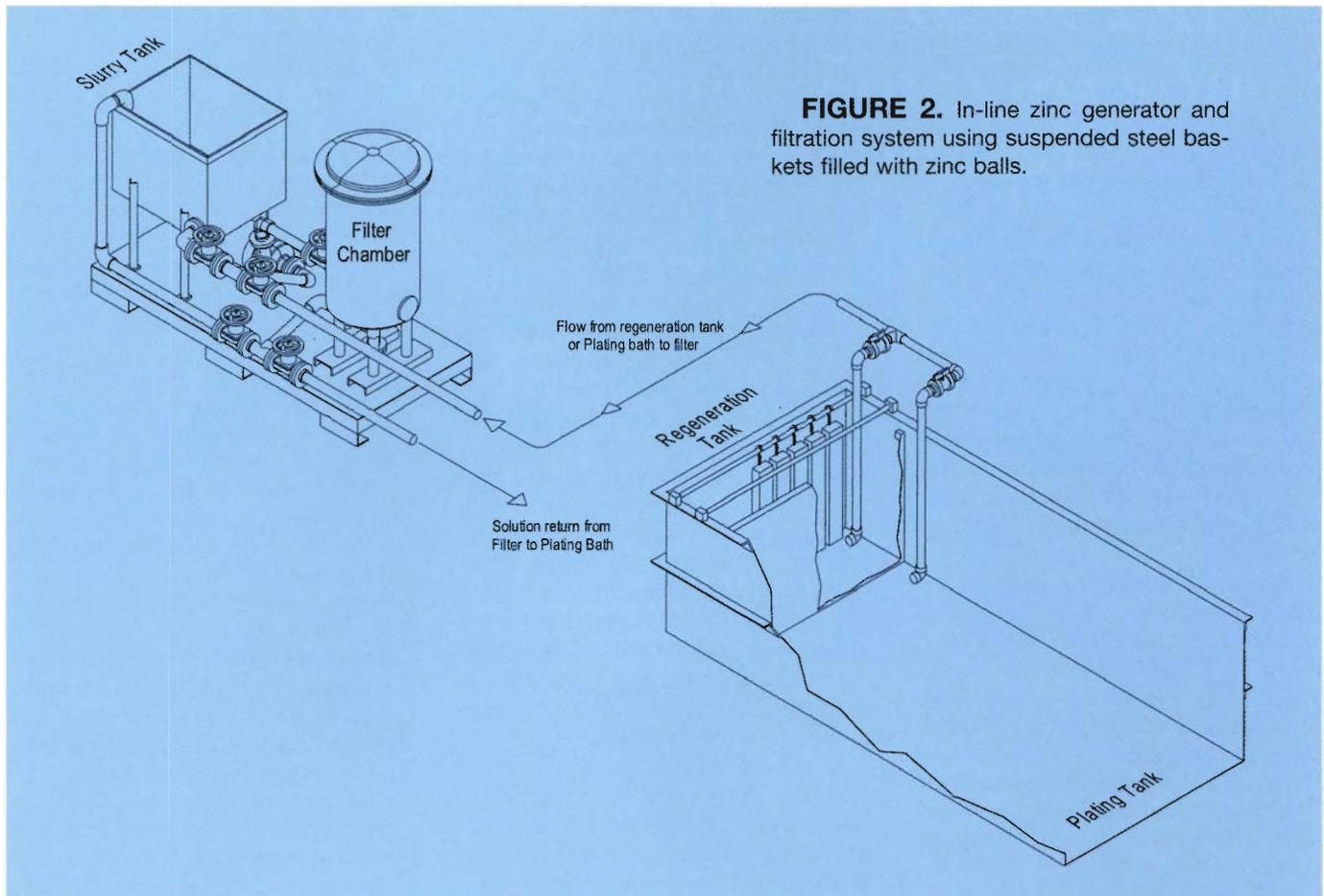
**FIGURE 2.** In-line zinc generator and filtration system using suspended steel baskets filled with zinc balls.
