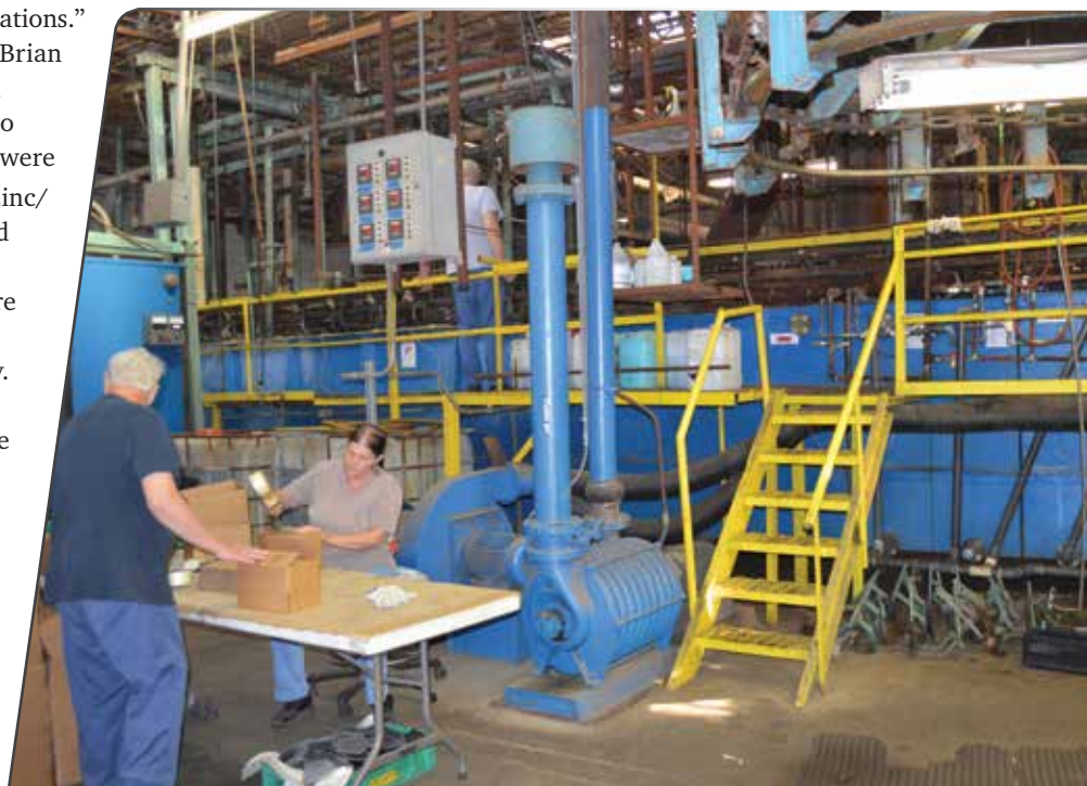
The zinc-nickel plating racks enable Micro Metal Finishing to plate parts up to 50 inches long and 15 inches wide.
