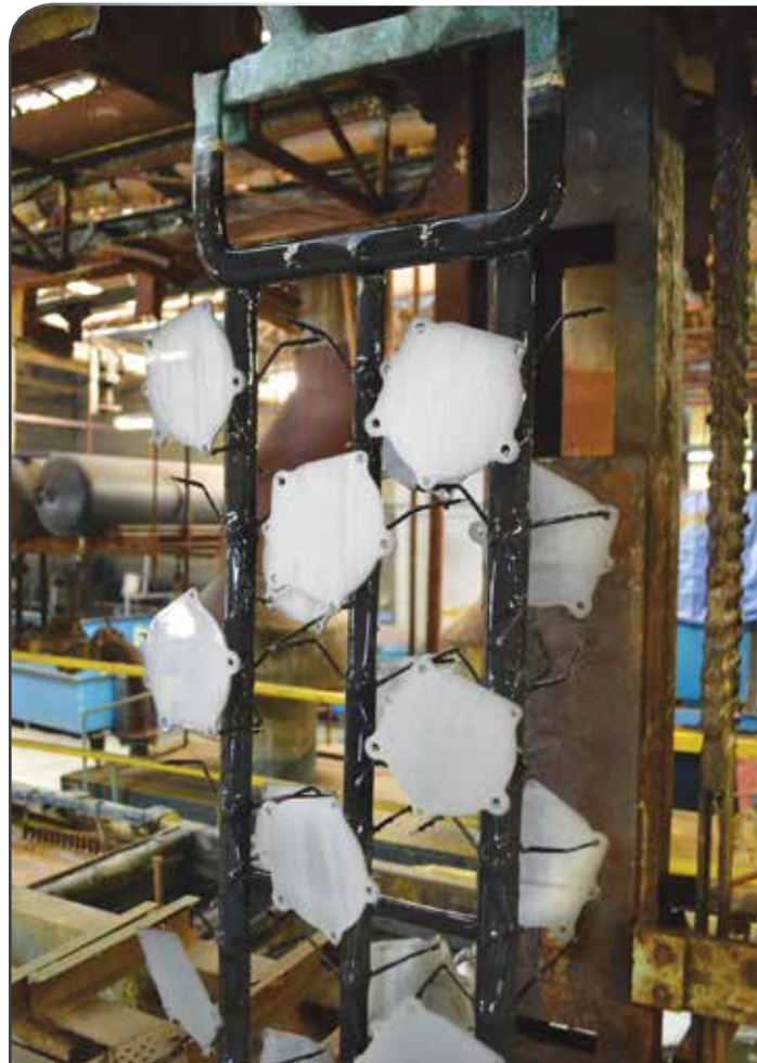
The zinc-nickel plating racks enable Micro Metal Finishing to plate parts up to 50 inches long and 15 inches wide.
