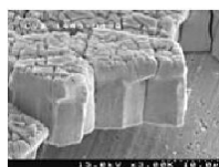
Figure 2 Laminar zinc deposit structure from acid chloride plating.
