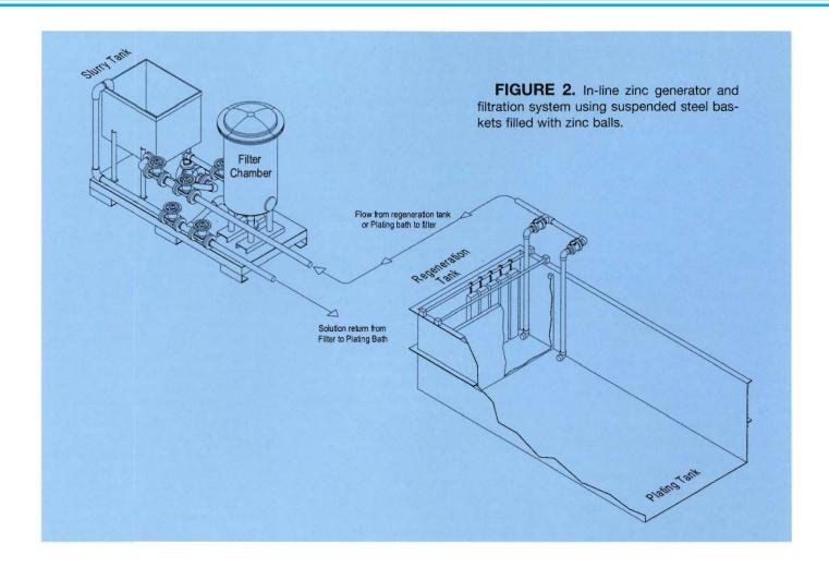
of the plating tank; some high-volume platers increase the size of the generator tank to around 33% in order to ensure adequate zinc reservoirs.
